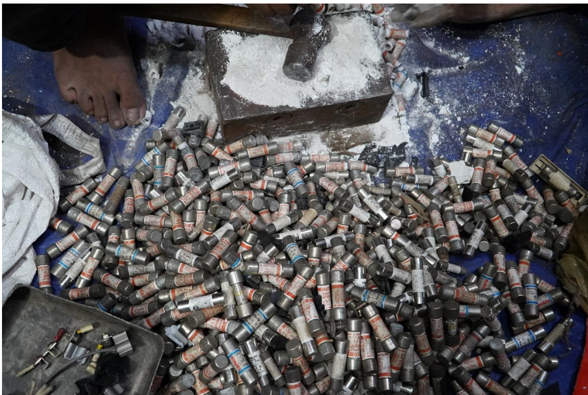
An informal dismantler separating fuses using a hammer without personal protective equipment.
